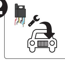
**PLACE THE ECU SOCKET IN THE ENGINE COMPARTMENT ON THE LEFT SIDE**
